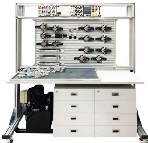
S/N F21841 (Electro Hydraulic Training Set)
